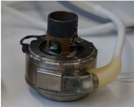
(left) The HeartMate 3 by Abbott with modified inflow cannula, (right) cannula with two embedded pressure sensors
